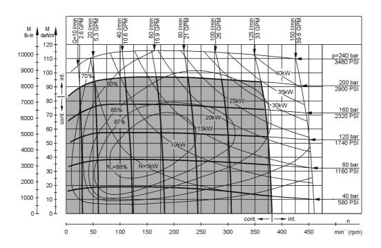
The function diagrams data is for average performance of randomly selected motors at back pressure 5÷10 bar [72.5÷145 PSI] and oil with viscosity of 32 mm²/s [150 SUS] at 50°C [122°F].
