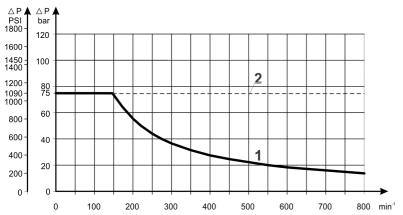
Curve "1" shows continuous operations. Curve"2" shows intermittent operations.
