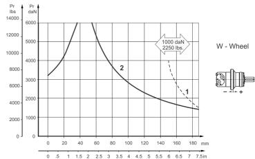
Curve "1" shows critical radial shaft load. The output shaft runs in tapered bearings that permithigh axial and radial forces. The permissible radial loadon the shaft is shown (curve 2) for an axial load of 0 Nas function of the distance from the mounting flange to the point of load application. The curve 2 apply to a B10 bearing life of 2000 hours at 100 RPM.
